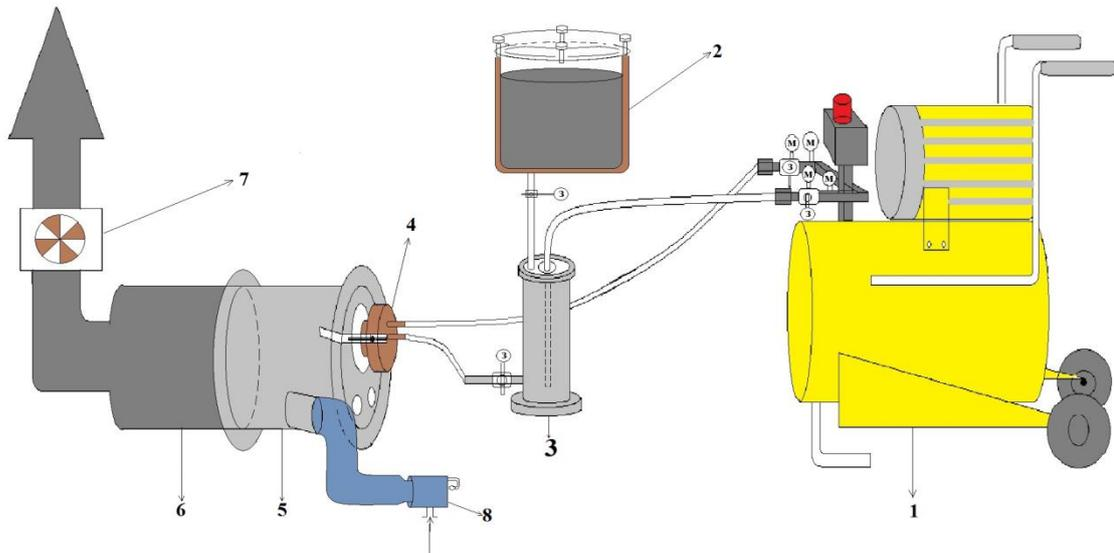
1- compressor, 2 – WCF storage tank, 3 – WCF tank, 4 – WCF nozzle, 5 – burner device, 6 – combustion chamber, 7 – blowing fan, 8 – ignition burner
