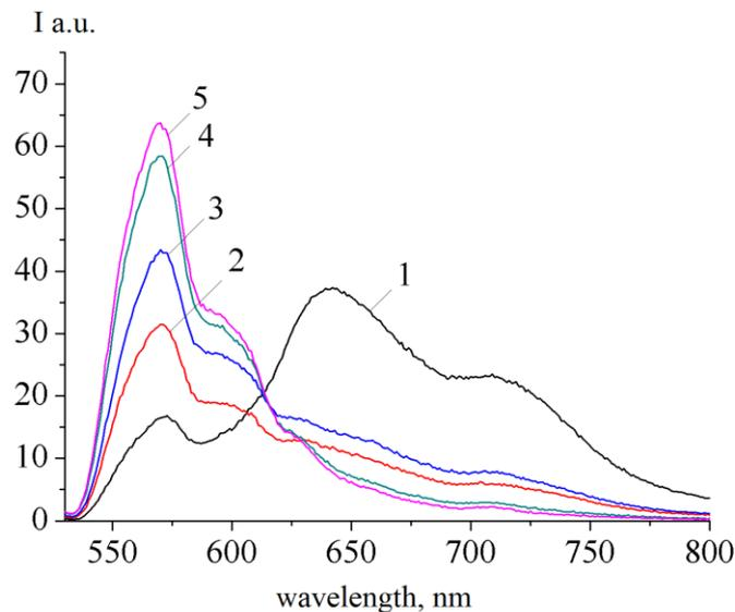
**Fig.4.** Fluorescence spectra of the films P3HT on the surface of the islet silver films obtained at different annealing temperatures: 1 – without NPs; 2 – 20 °C; 3 – 120 °C; 4 – 180 °C; 5 – 240 °C.
