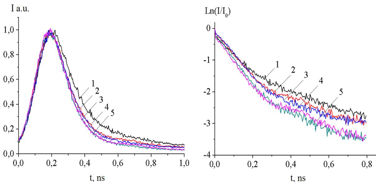
**Fig.5.** The kinetics of fluorescence decay P3HT films on the surface of the islet silver films: 1 – without NPs; 2 – 20 °C; 3 – 120 °C; 4 – 180 °C; 5 – 240 °C.
