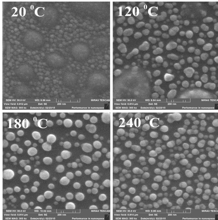
**Fig.1.** SEM image of the islet silver films on a solid substrate which were obtained with different annealing temperatures.
