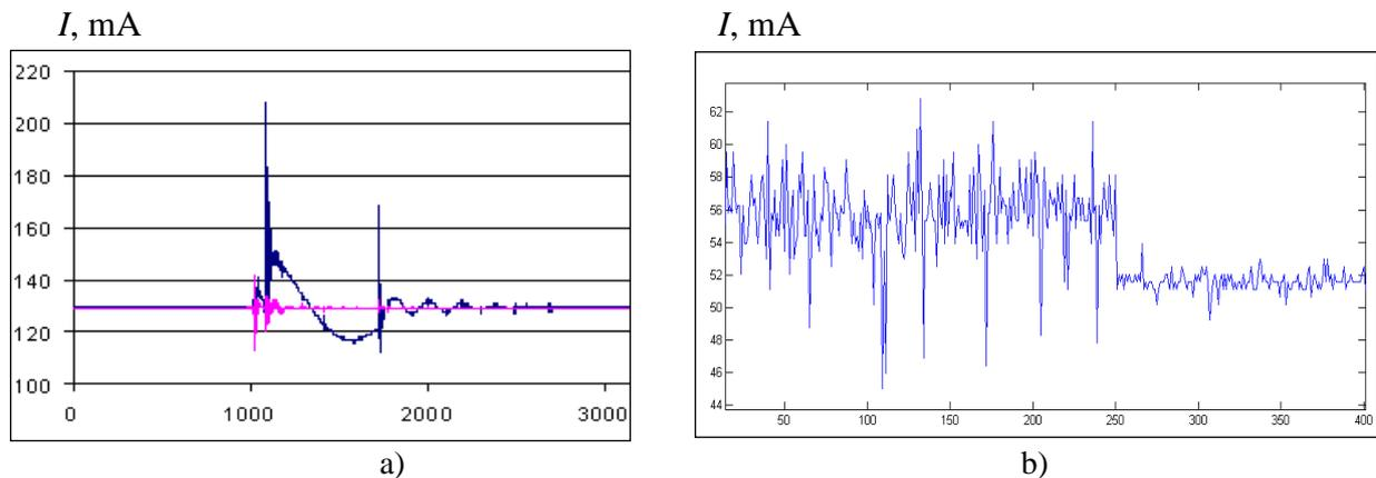
**Fig.4.** Current oscillograms at: a) – single and b) – repeating electrical discharges of a preset frequency.
