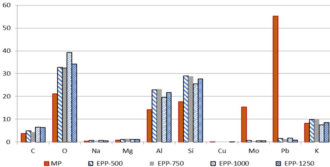
**Fig. 8.** Change in elemental composition in samples of technogenic raw materials from the Annensk mine after processing: mechanical processing (MP); electric pulses processing (EPP).
