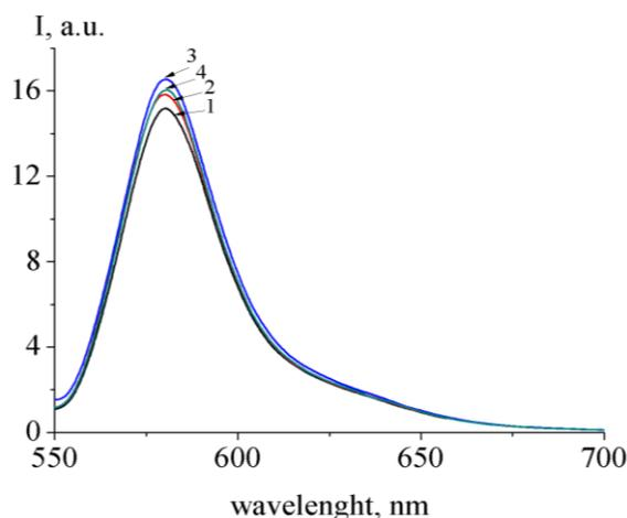
Fig.4. Effect of Au nanoparticles on Rhodamin C fluorescence in ethanol:
