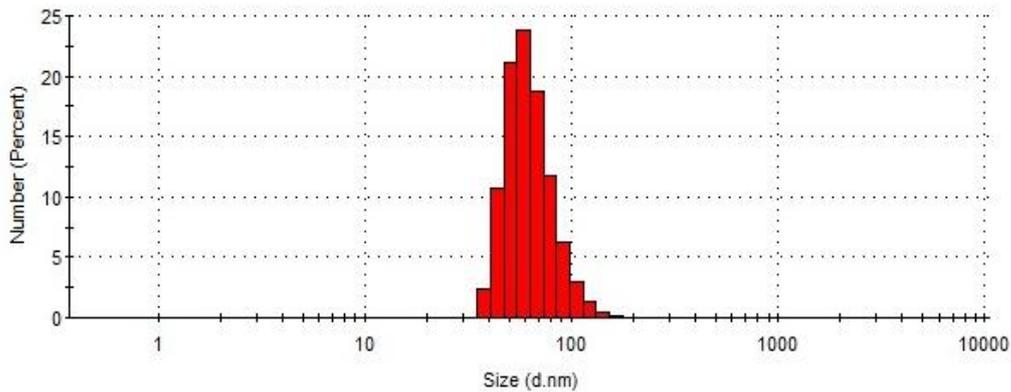
Fig. 1. The average sizes of Au nanoparticles
