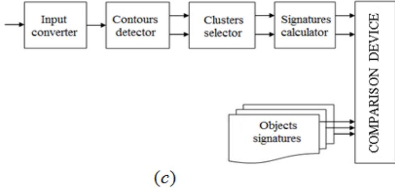
Fig.5. The initial (a) and detailed (b, c) structures of the first fractal detectors.
