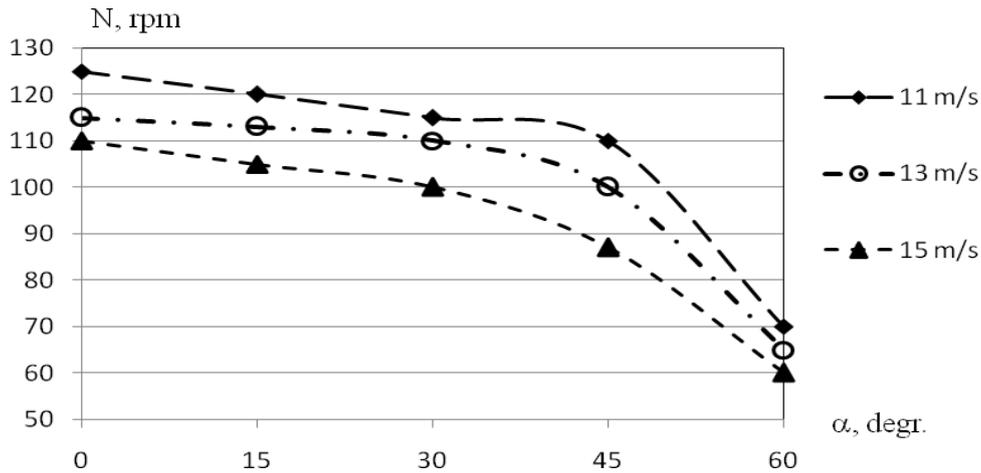
Fig.4. Dependence of rotation frequency on the yaw angle of the flow  $\alpha$  at three different flow rates
