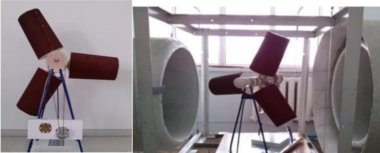
Fig.1. The model of the wind turbine with rotating cylinders of various cross-sections:
