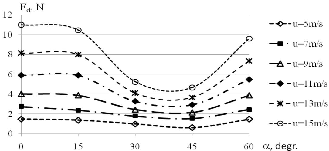
Fig.3. Dependence of the drag force on the yaw angle of the flow  $\alpha$  at different flow rates.
