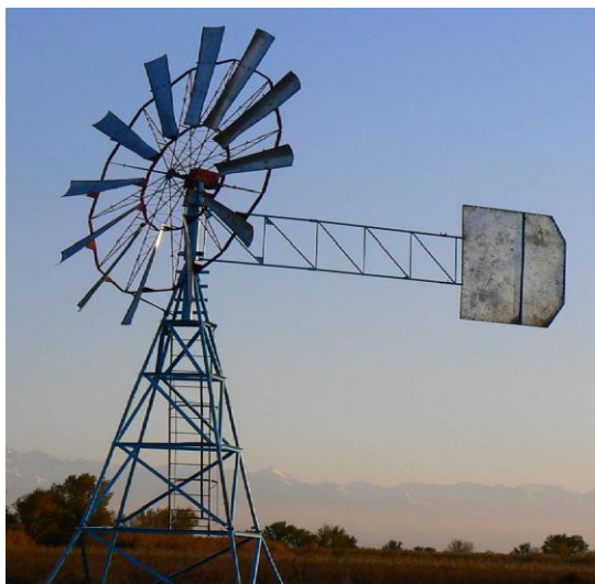
Fig.8. Slow multi-bladed installation of Kazakh Research Institute of Mechanization and Electrification of Agriculture
