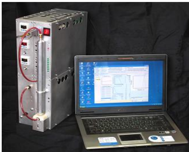
Fig.1. The outside appearance of the aerosol diffusion spectrometer
