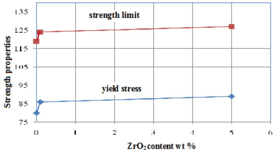
Fig. 2. Strength characteristics change depending on the amount of ZrO<sub>2</sub> filler
