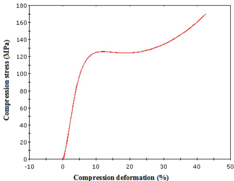
Fig. 3. Deformation curve of the PMMA sample containing 0,1% ZrO<sub>2</sub> at a static compression test
