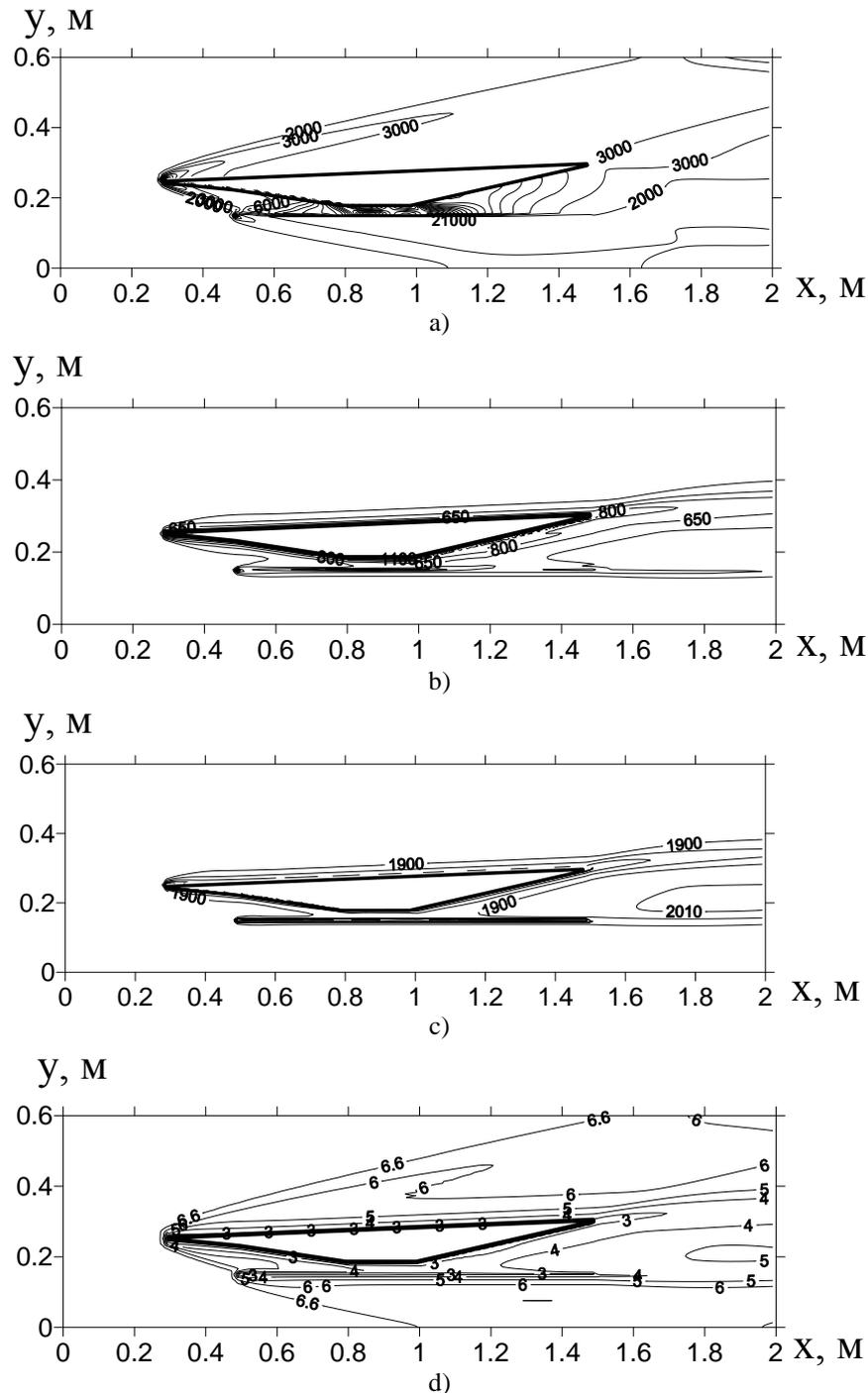
Fig. 2. Fields of pressure, in  $pa$  (a), temperature (K) (b), horizontal velocity(m/s)(c), and the Mach numbers (d) in the flow of air and combustion products in the scramjet channel. The incoming flow velocity was  $U_0 = 2000$  m/s, and the mass supply rate of the fuel (hydrogen) was  $G\Sigma H_2 = 0.01$  kg/(s · m).
