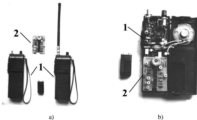
Fig. 3. The pilot radiofrequency band transmitter-receiver device using chaotic signals: a) the exterior view of the transceiver (1); b) a chaotic module (2) built in the transceiver
