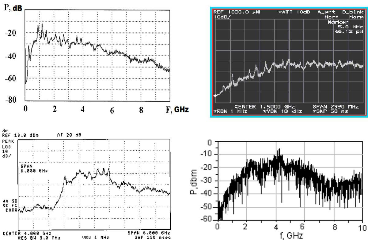
Fig. 1. Examples of power spectra of the output signals of different chaos generators.
